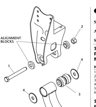
**IMPORTANT:** Different frame widths require various spacer washer placement at the pivot connection.
